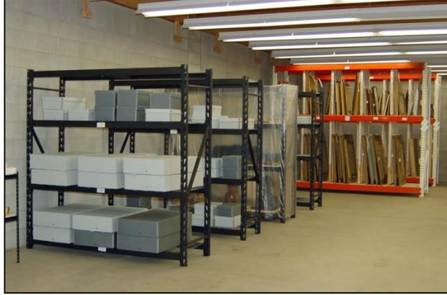
For the large or heavy objects, we reinforced the  $\frac{3}{4}$  inch plywood shelves with stringers spanning the beams. (I selected the 48 inch deep shelves for more versatility.) Make sure the wood stringers are screwed to the shelf and fit the depth of the inset of your pallet racking beams. I also use unbleached muslin cut to size as a dust cover for each object.
